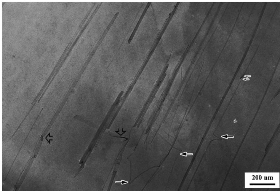
**8 Alignment of nanotubes in polymer matrix following cutting with microtome: arrows indicate buckled nanotubes<sup>39</sup>**
