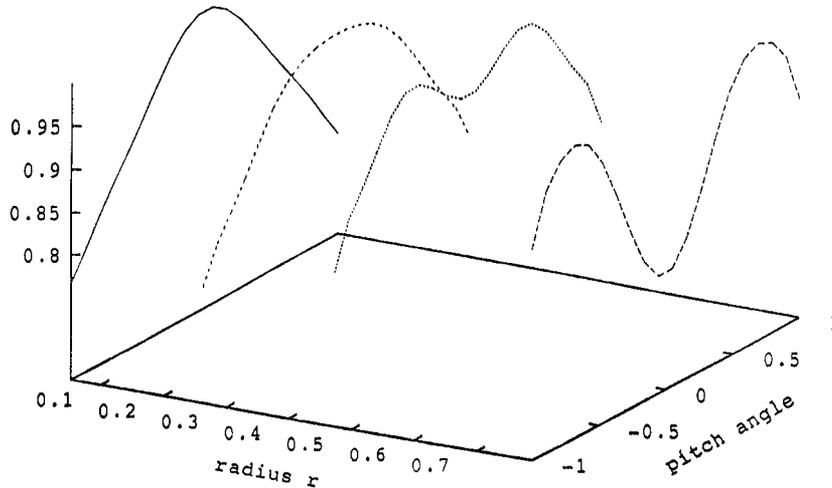
FIG. 9. The dependences of the fast electron distribution  $f/f_0$  on  $\mu$  at various positions over the radius;  $dB/dr < 0$ .
