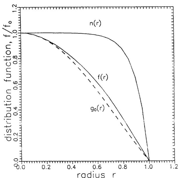
FIG. 3. The distribution over the discharge of the initial density profile  $\bar{n}(r)$ , the distribution function  $f(r)$  at  $y = 1$ , obtained in solving the system (16) and the eigenfunction of the problem (12) (dashed line).
