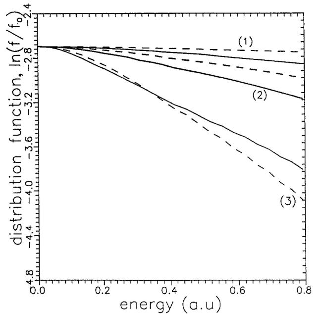
FIG. 8. The dependences of the fast electron distribution function  $\ln(f/f_0)$  on longitudinal (solid line) and transverse (dashed line) energy, in the presence of a finite mean magnetic field gradient: (1)  $dB/dr > 0$ , (2)  $dB/dr = 0$ , (3)  $dB/dr < 0$ .  $r = 0.95$ .
