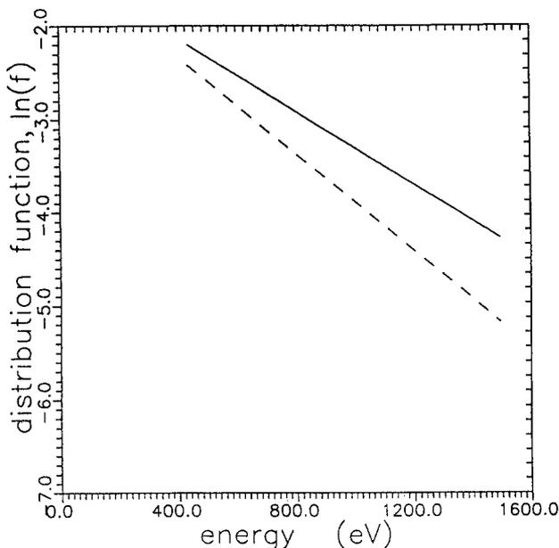
FIG. 14. The dependences of the fast electron distribution function  $\ln(f)$  on longitudinal (solid line) and transverse (dashed line) energies for particles moving along the magnetic field line;  $\beta = 0.17$ ,  $\delta_1 = 0.21$ ,  $\delta_2 = 0.036$ .
