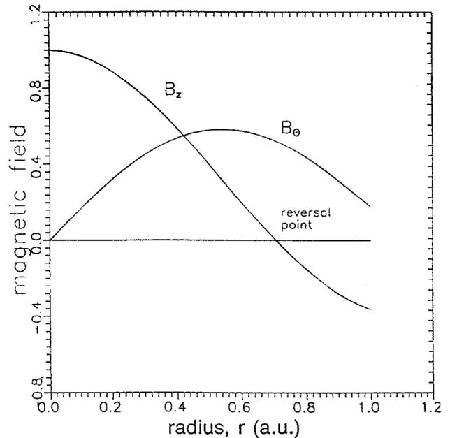
FIG. 10. The radial distribution of magnetic field components along the minor radius.
