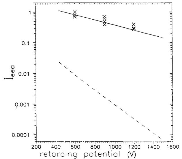
FIG. 11. Comparison of theoretical versus experimental current  $I_{eea}$ , collected by an electron energy analyser as a function of the retarding potential  $V$  for the case of ZT-40M. The solid line is for particles moving along the magnetic field line and the dashed line for particles moving backward. The experimental data are shown by labels.
