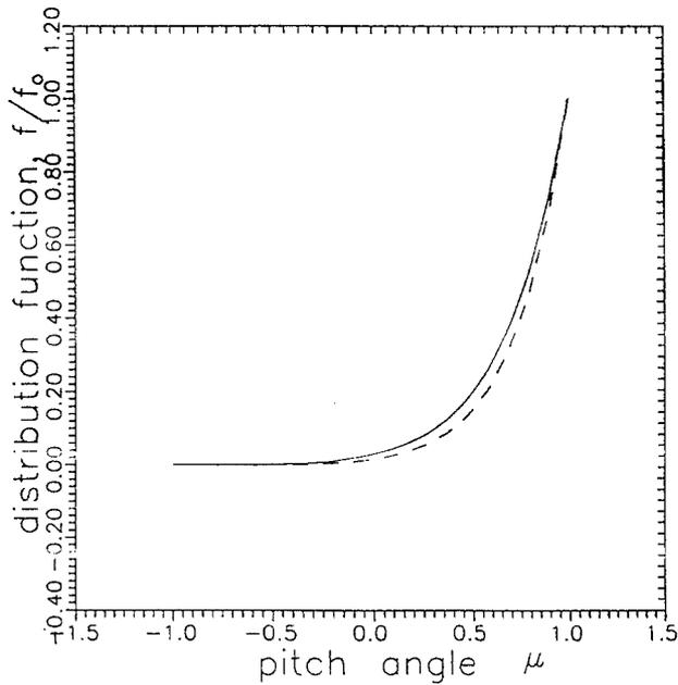
FIG. 6. The fast electron distribution function  $f/f_0$  as a function of  $\mu$  with an applied electric field  $E_e$  present. The solid line is the polynomial solution at  $y > 1$  and the dashed line is the exponential solution at  $z = y\delta_2^{1/2} \ll 1$ .
