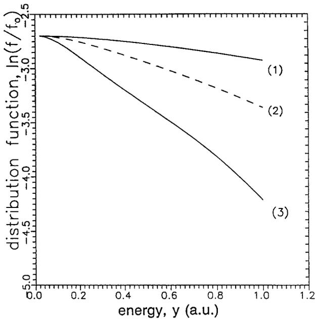
FIG. 7. The dependences of the fast electron distribution function, averaged over  $\mu$ ,  $\ln(f/f_0)$  on energy  $y$  with a finite mean magnetic field gradient present: (1)  $dB/dr > 0$ , (2)  $dB/dr = 0$ , (3)  $dB/dr < 0$ .  $r = 0.95$ .
