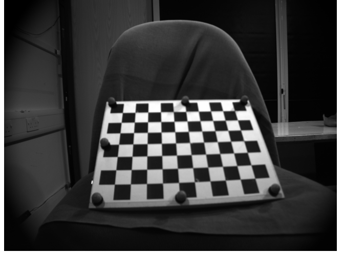
Fig. 3: Image of Tsai grid captured by the camera.
